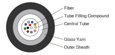
Note: Drawing is the 12 Fibers cable as example
